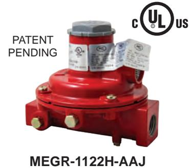
**MEGR-1122H Series:** Offers a compact first stage regulator design perfect for tight applications such as underground tank domes. They feature an adjustment range from 9-12 PSIG (factory set @ 10 PSIG), stainless steel internal components, fluorocarbon (FKM) seat discs, molded lip fabric reinforced diaphragms and large aluminum precision machined orifice to minimize freeze ups while providing superior downstream regulation and maximum corrosion resistance against weather or contaminated gas.
